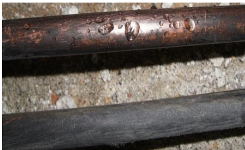
Damaged hydraulic hose pipe
